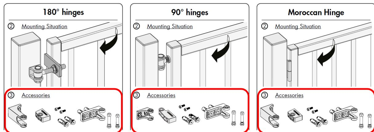
Selecting the wrong accessories may reduce the closing force or completely prevent the gate closer from working properly.
