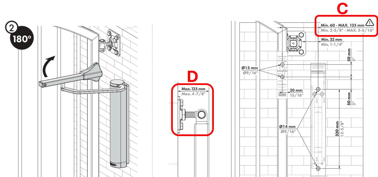
C - Distance between gate closer middle position to rail fixation hole (mm):
