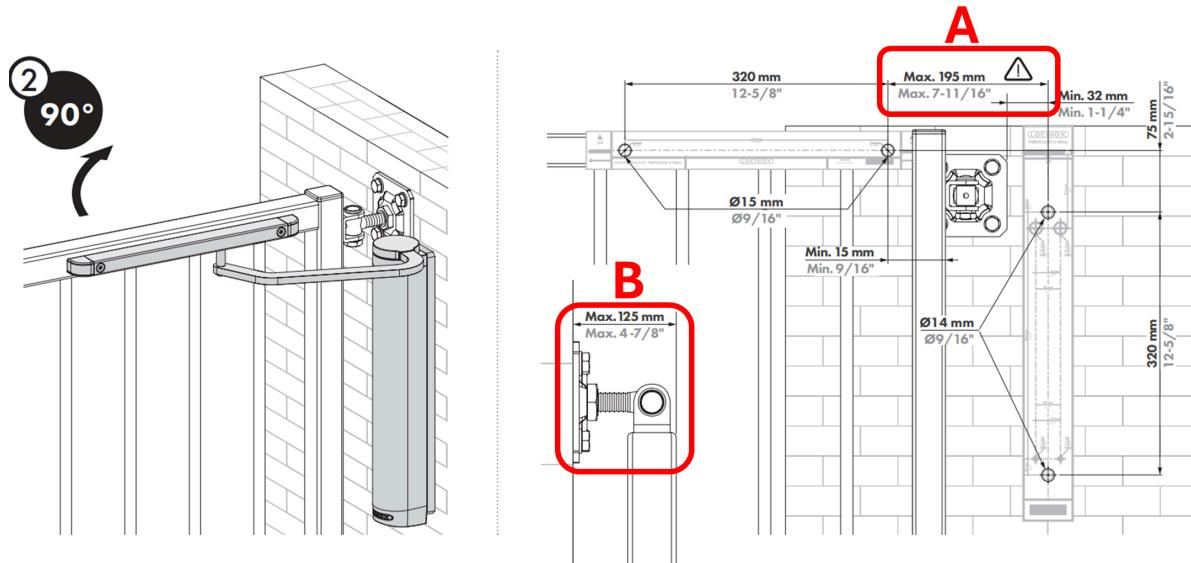
A - Distance between gate closer middle position to rail fixation hole (mm):
