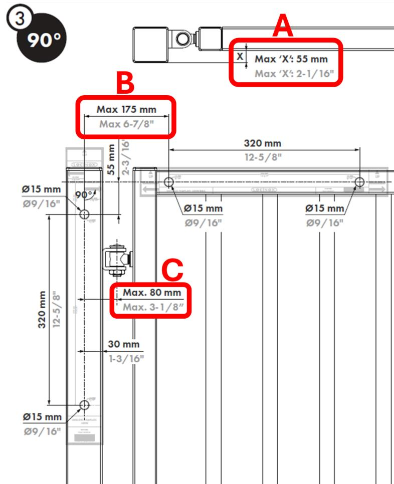
A - Distance between edge of the post to gate frame (mm):
