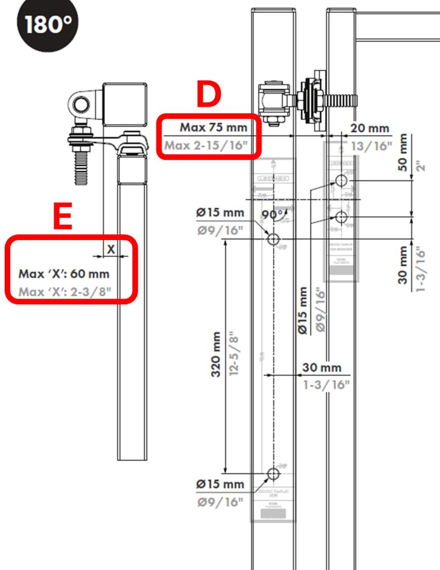
D - Distance between post profile to the gate frame (mm):
