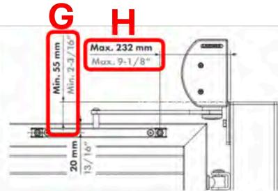
H - Distance between Panther adaptor plate to first rail fixation hole (mm):
