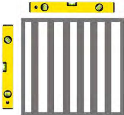
Please check that the gate is properly installed **using a spirit level**. Uneven installation reduces the effectiveness of the gate closer.
