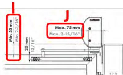
J - Distance between Panther adaptor plate to first rail fixation hole (mm):
