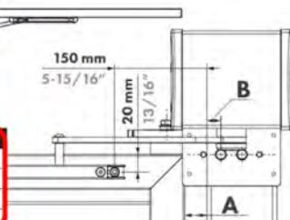
B - Distance between edge of the post profile and first fixation hole closer to this edge in (mm):
