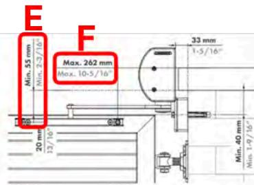
F - Distance between Panther adaptor plate to first rail fixation hole (mm):
