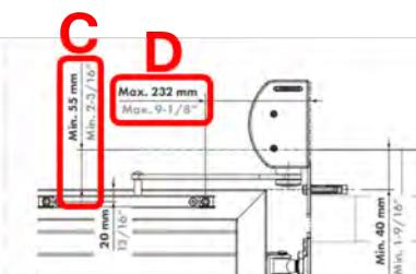
C - Distance between top edge of the post to gate frame (mm):
