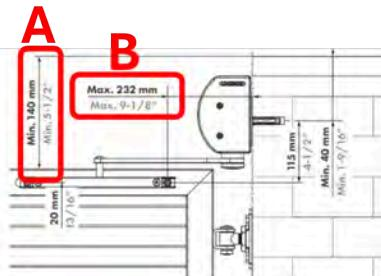
A - Distance between top edge of the post to gate frame (mm):
