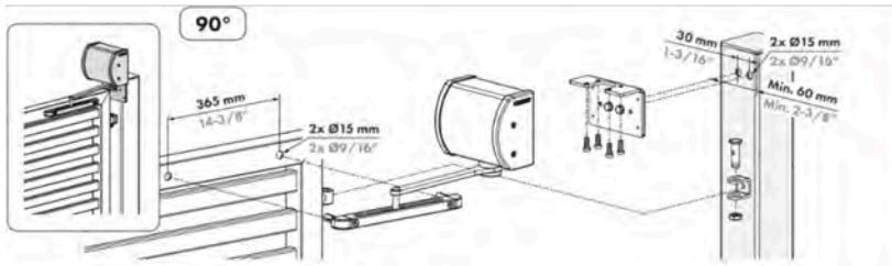
G - Distance between top edge of the post to gate frame (mm):
